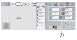
① The threads threaded on the needle bars are indicated as shown here.
